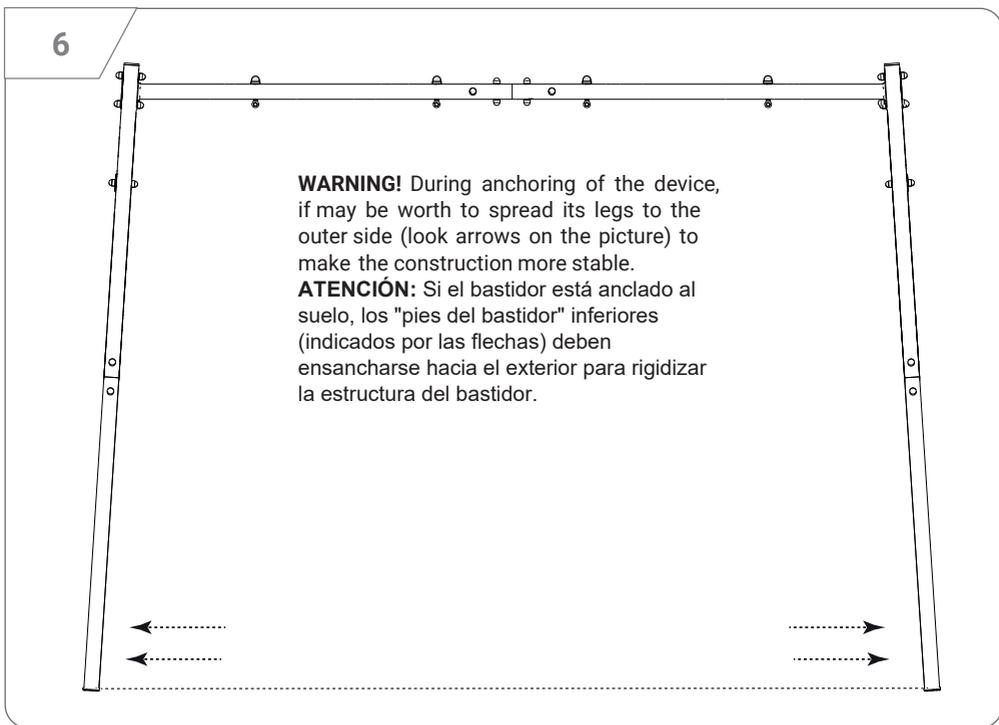
**WARNING!** During anchoring of the device, if may be worth to spread its legs to the outer side (look arrows on the picture) to make the construction more stable.
