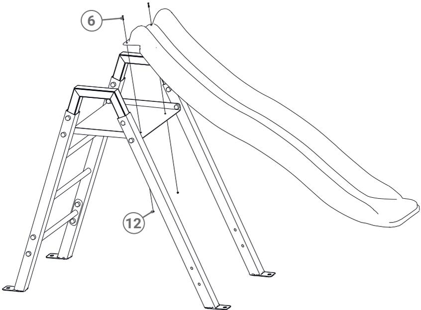
**ENG:** The slide operates as a separate element. It can be additionally attached to the swing by removing the appropriate screws to join the frames using the metal connector no. 14. If you do not wish to do this, skip this step.
