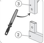
**NOTE:** During the installation of the device, it may be necessary to file the internal side of profiles into which profiles with smaller dimensions are inserted.
