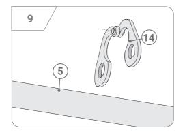
To prevent movement of the clamp, place a piece of a rubber between the rod and the clamp.
