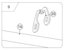
To prevent movement of the clamp, place a piece of a rubber between the rod and the clamp.
