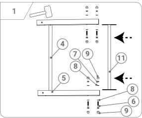
If you find it difficult to fit the pipe inside the opening, use hammer to shorten the diameter of the pipe by 1 mm.
