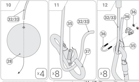
The length of the metal ropes should allow the weight to lay easily on the metal profiles meanwhile, the round rubber bumpers should be as close as possible to the part number 3.
