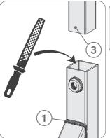
**NOTE:** During the installation of the device, it may be necessary to file the internal side of profiles into which profiles with smaller dimensions are inserted.
